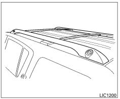
The crossbars can be adjusted forward and backward. Loosen the thumbwheel (1) and adjust the crossbar to the desired position. Tighten the thumbwheel. Place your luggage on the bars and secure the luggage with rope to the utility loops (2). Do not place luggage on the side rails or tie rope directly to the side rails. Always be sure the thumbwheels are fully tightened to keep the crossbar in place. Do not use utility loops for any purpose other than securing luggage.
